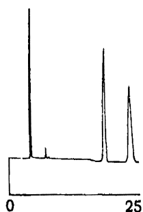
Fig. 4. Chromatographic separation of \alpha -phenylethanol. Column temperature=150°C. Time scale in min.
